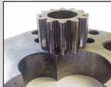
Cast iron material torn away from case bore and "welded" to the tips of the gear teeth (adhesive wear)
