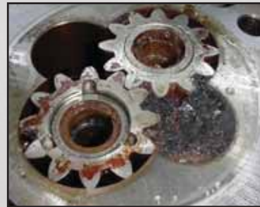
Gears seized by buildup of rust products
