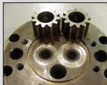
Galling damage to a cast iron faceplate
