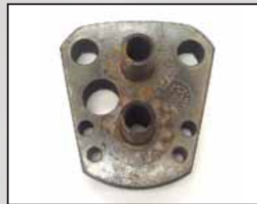
Rusted cast iron faceplate from a circular flow divider
