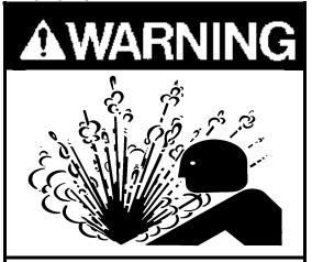
Over-pressure may burst pump or system components. Always include a relief valve in installation. Do not over pressurize pump or block discharge line while running.
