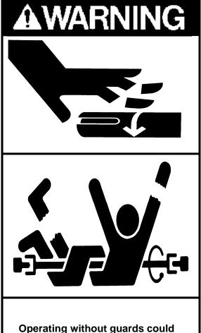
Operating without guards could result in serious injury or death. Machinery in operation can grab, crush, cut, mangle and dismember. Do not operate without adequate guards in place.
